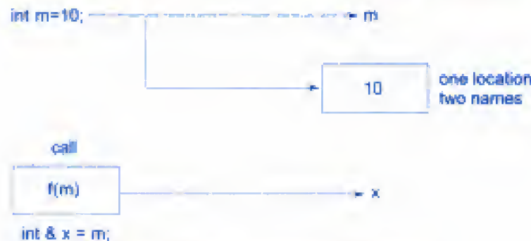
Fig. 3.2 ⇒ Call by reference mechanism
